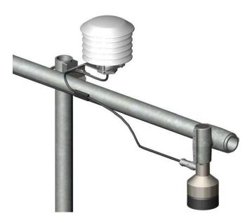
This configuration includes an SR50A attached to a crossarm via the 19484 mounting stem and a NU-RAIL fitting. A 107 temperature probe housed in a 41303-5A 6-Plate Gill Radiation Shield provides the air temperature measurement.
